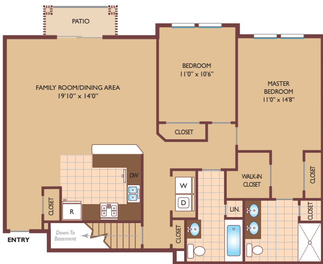
Manor Home - Module "B" Two Bedroom Floor Plan with 2 Bath, 1,243 sq. ft. First Floor
